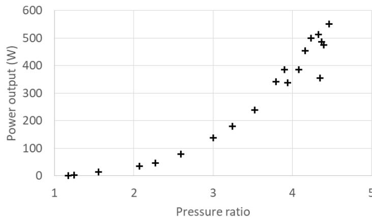
Figure 3. Electrical power produced as a function of the measured pressure ratio
