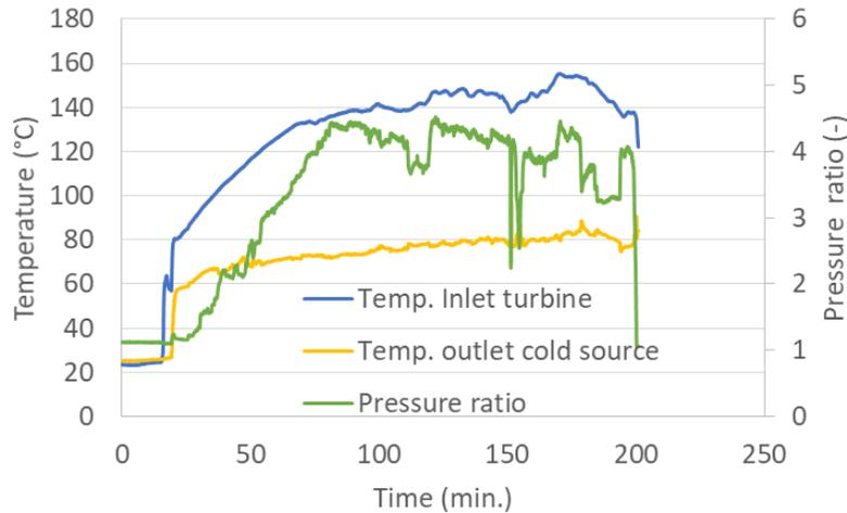
Figure 2. Temperature and pressure ratio obtained during on-site tests
