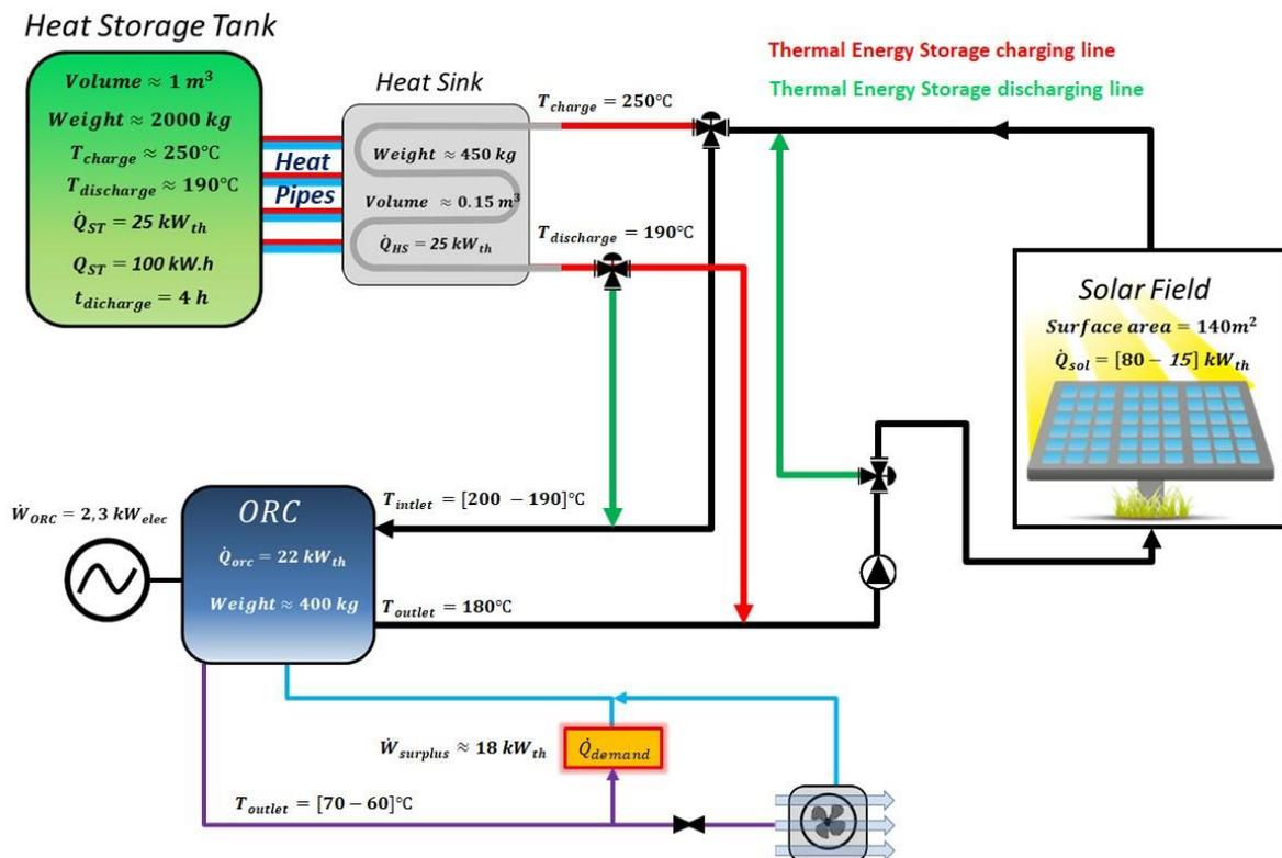
Figure 1. S-ORC system architecture
