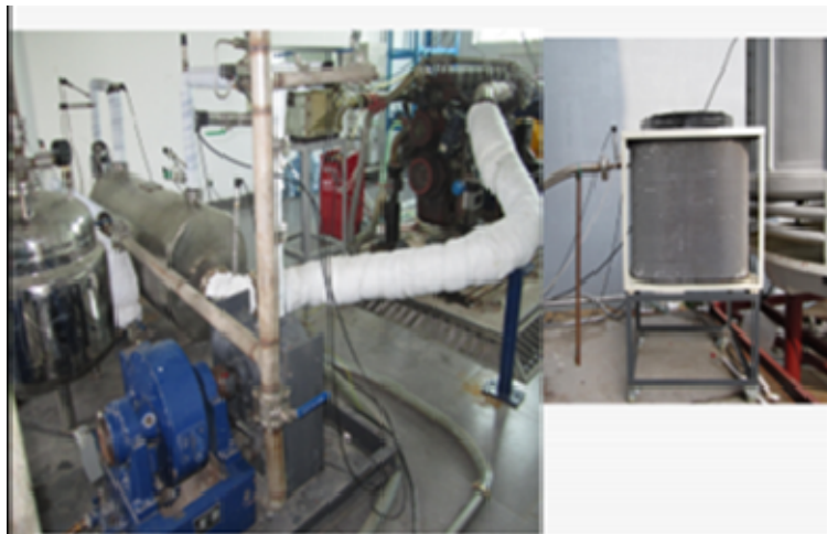
Fig.11: ORC demonstration projects from diesel Engine waste heat [18]
