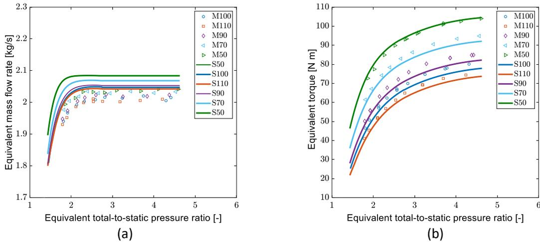
**Figure 1.** Comparison of AxialOff with the single-stage turbine in Kofskey and Nusbaum (1972).
