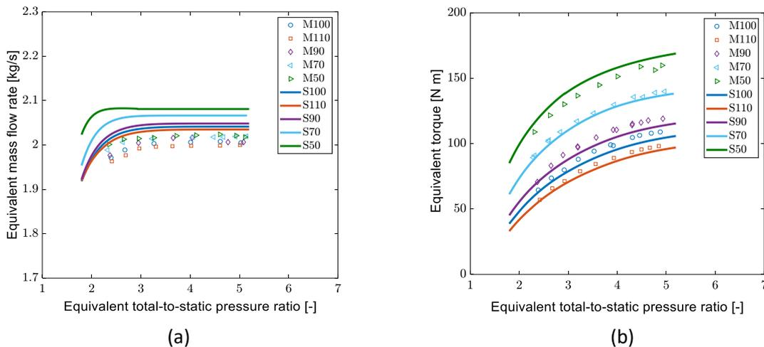
**Figure 2.** Comparison of AxialOff with two-stage turbine in Kofskey and Nusbaum (1972).
