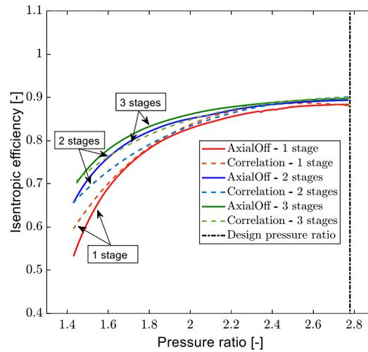
Figure 3. Comparison of performance map of R245fa turbine between AxialOff and part-load correlations.
