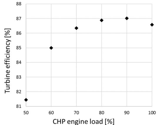
**Figure 10:** Calculated isentropic turbine efficiency (total to total) of the turbine (simulation results)
