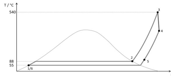
Figure 3: T-s-diagram of the SRC
