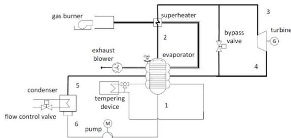
Figure 4: Flow diagram of the SRC plant
