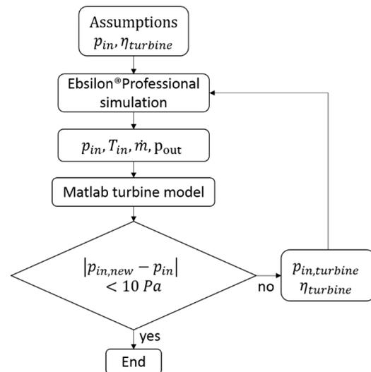
**Figure 6:** Calculation of the evaporation pressure and the turbine efficiency in the simulation
