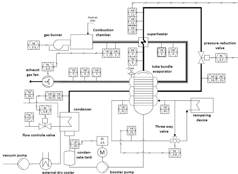
Figure 7: Flow diagram of the test rig with measuring devices
