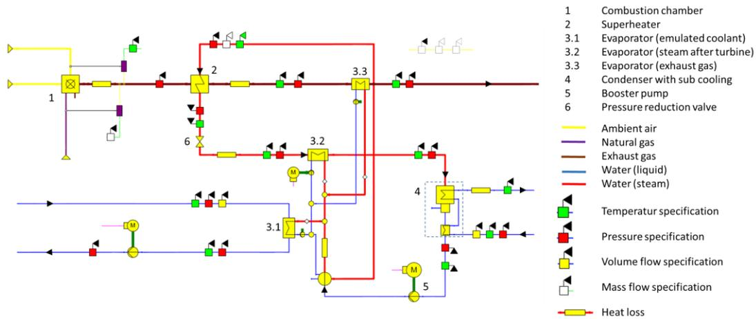
Figure 5: Ebsilon® Professional model for thermodynamic simulation and measuring data reconciliation
