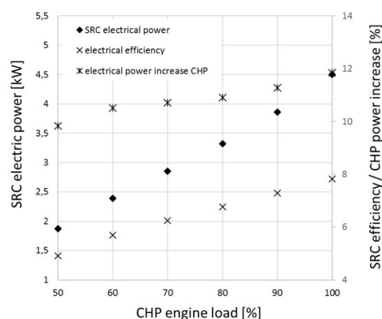
**Figure 9:** Electric power prediction of the SRC (calculated by the simulation model, extended by the turbine model)
