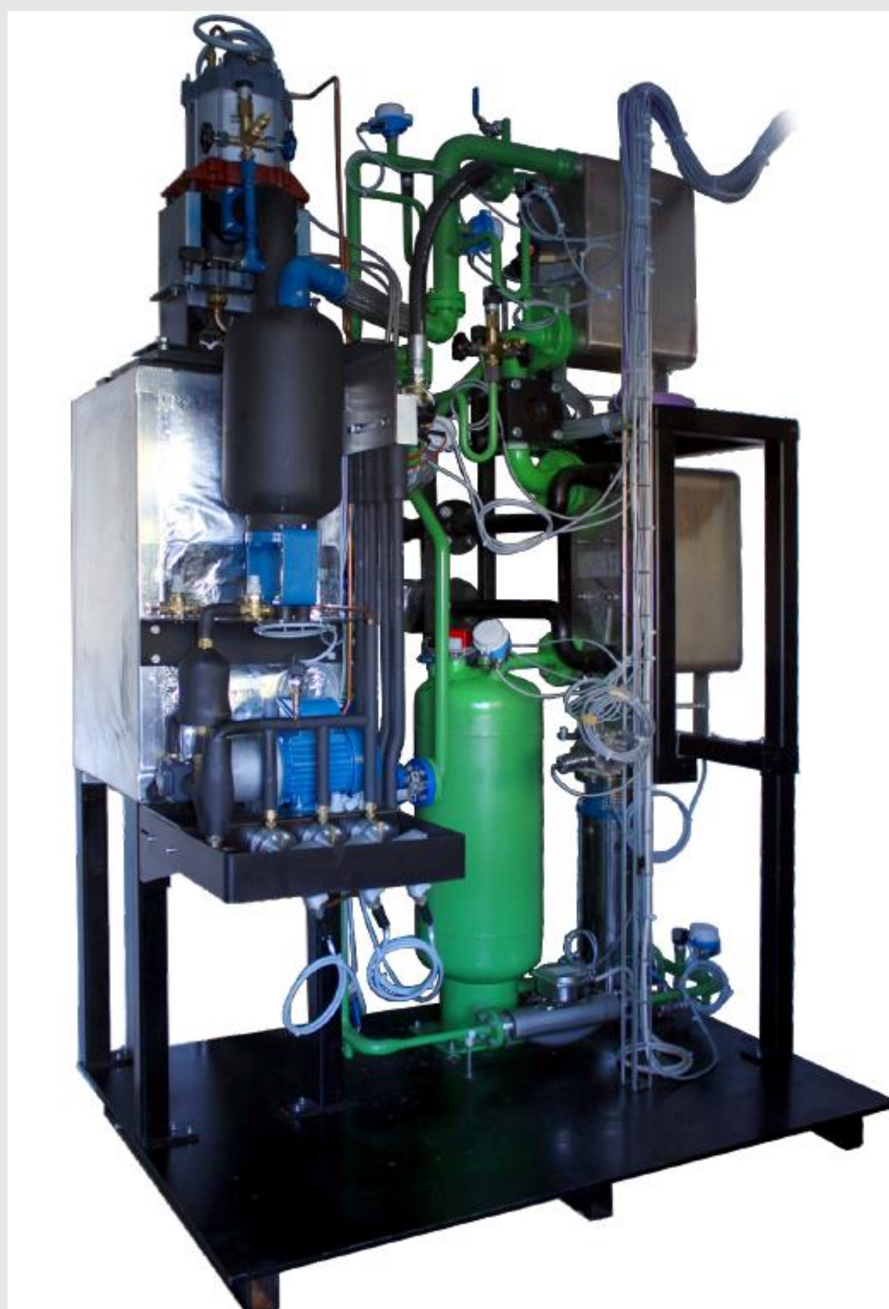
Figure 2. Picture of the experimental 11 kW ORC (campus Kortrijk Ghent University).
