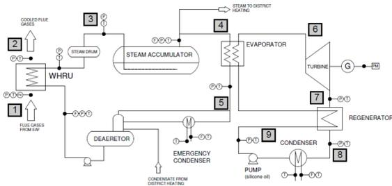
Figure 1. e-Recovery power plant flow diagram.
